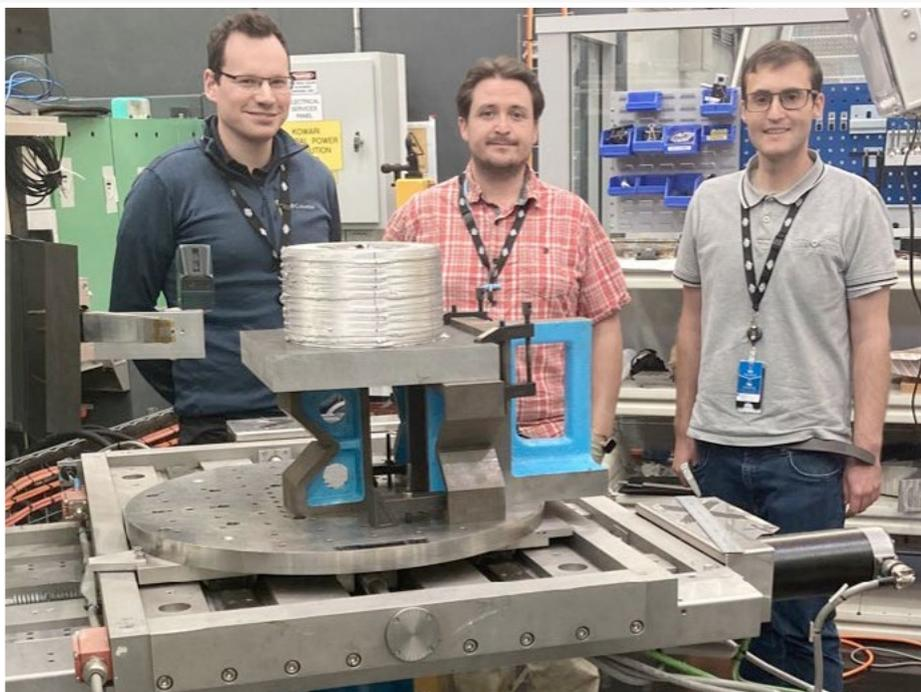
*Residual Stress Measurement of Additive Friction Stir Deposition on aluminium components on the Kowari Strain Scanner at ANSTO – Research team, University of Sydney*
