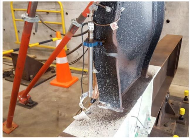
*HERA Seismic Research Programme, low cycle fatigue testing of a welded moment resisting frame connection at the University of Auckland, New Zealand [104]*
